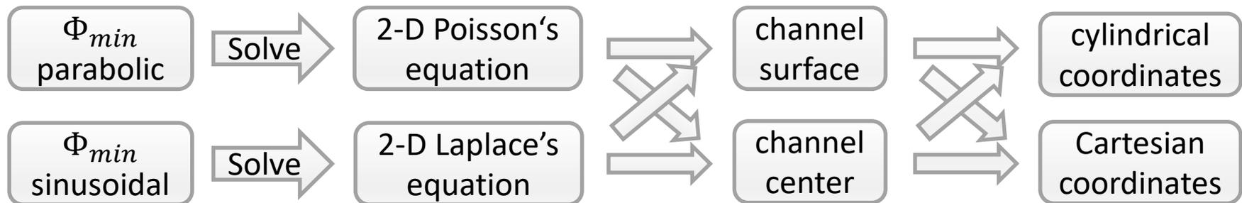
Equate the potential drops  $\Phi_{min}(r) = \Phi_{min}(x)$  and compare the potential drops along the channel  $\Phi(r, z) \propto e^{\pm z/\lambda}$  with the so-called natural length  $\lambda$  [4,5,6].
